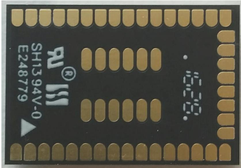
Figure 3: WGM110 External Photo, Bottom View
