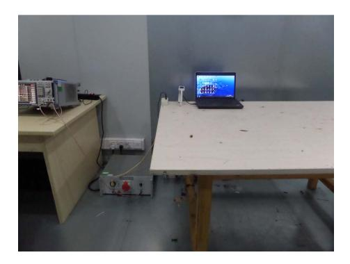
Radiation Emission Test Setup (Below 30MHz)
