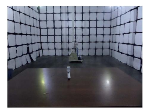
Radiation Emission Test Setup (Above 1GHz)
