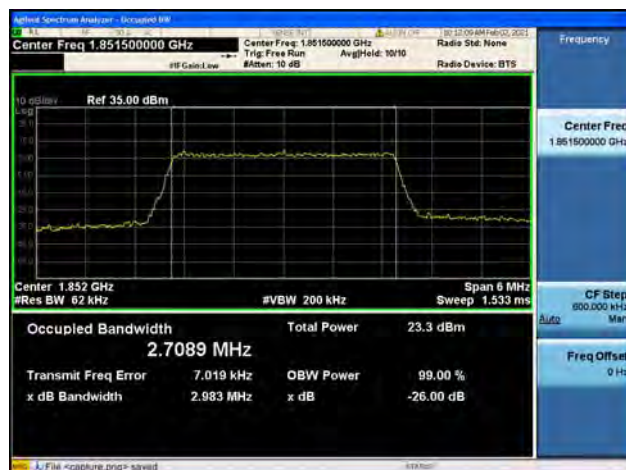
Band2 / 3MHz / Low CH / 16QAM
