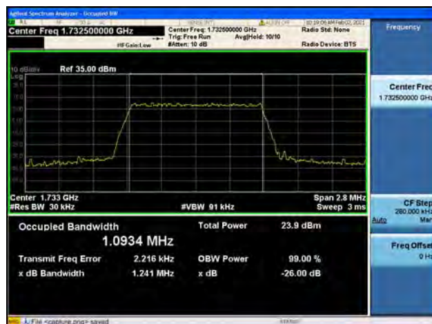
Band4 / 1.4MHz / Mid CH / 16QAM
