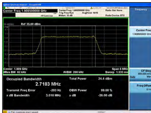
Band2 / 3MHz / High CH / 16QAM
