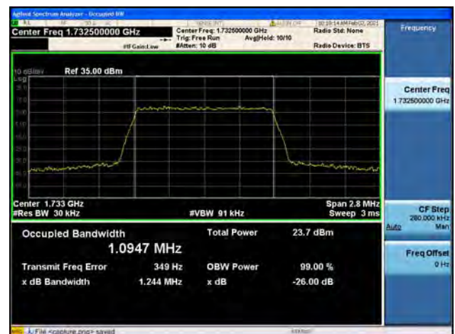
Band4 / 1.4MHz / Mid CH / 64QAM
