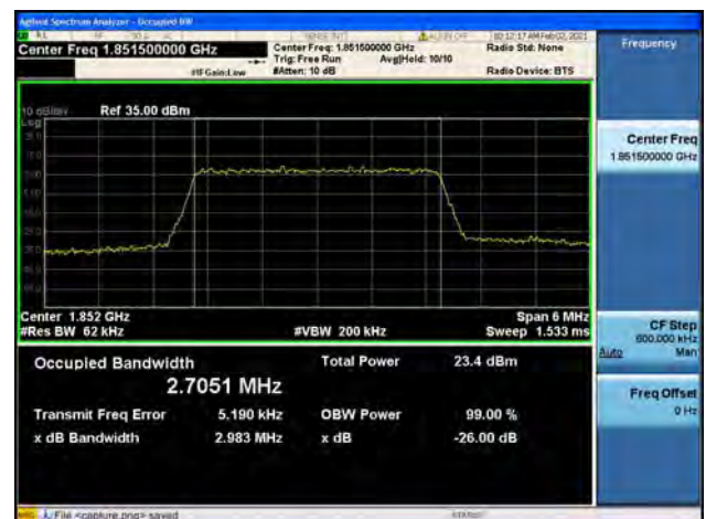
Band2 / 3MHz / Low CH / 64QAM
