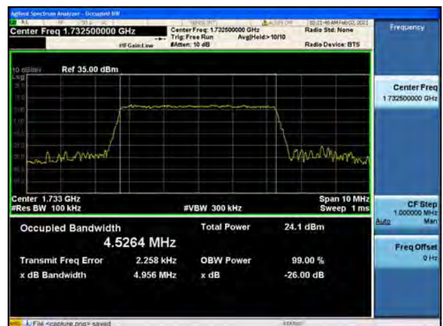
Band4 / 5MHz / Mid CH / 64QAM
