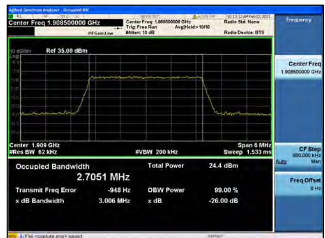
Band2 / 3MHz / High CH / 64QAM
