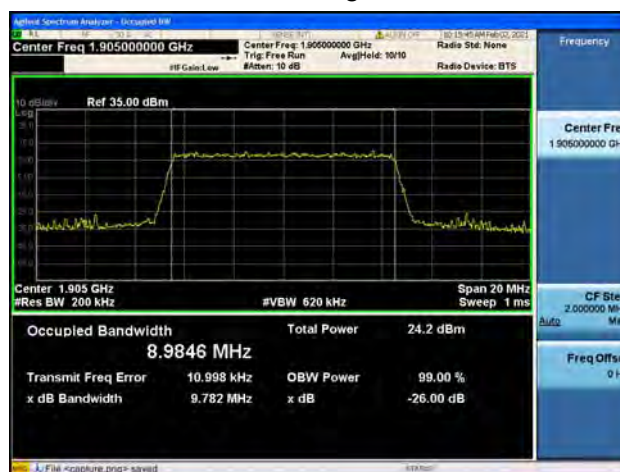
Band2 / 10MHz / High CH / 64QAM
