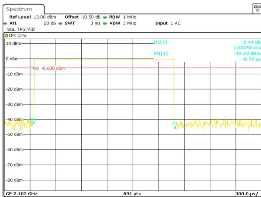
**Pulse time, Middle Channel, DH3**
