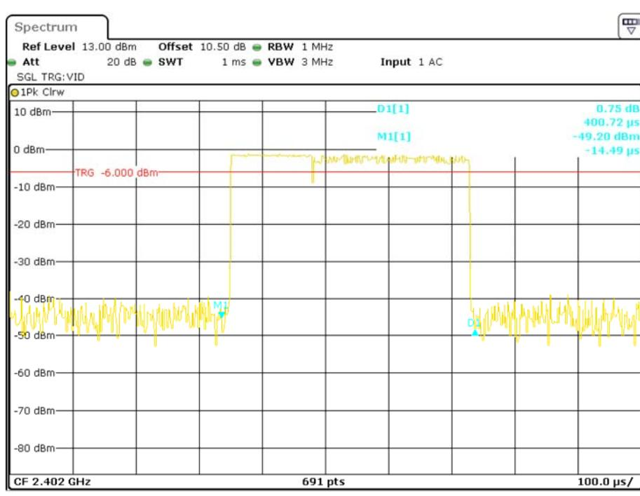
**Pulse time, Middle Channel, 2DH1**
