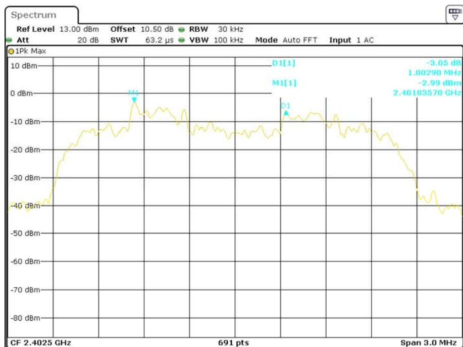
**EDR ( $\pi/4$ -DQPSK): Middle Channel**
