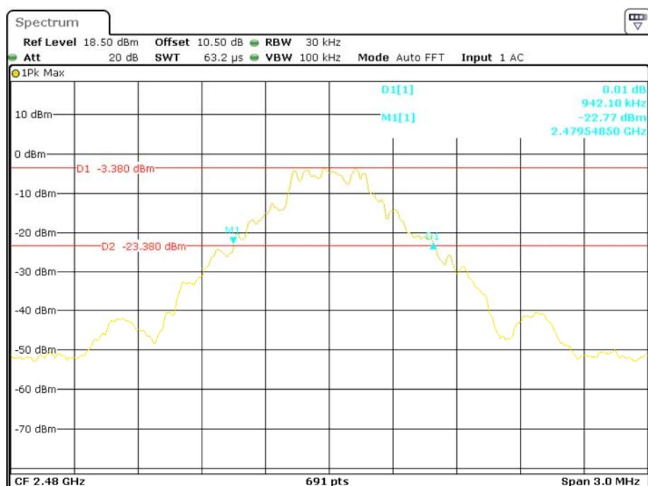
**EDR ( $\pi/4$ -DQPSK): Low Channel**
