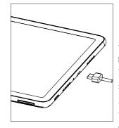
2. Open the slot and insert the SD card.
