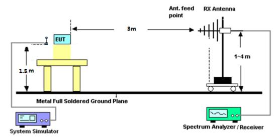
For radiated test from above 1GHz
