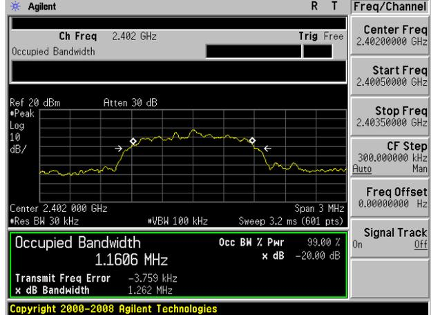
20dB Bandwidth plot on channel 39 (1Mbps)
