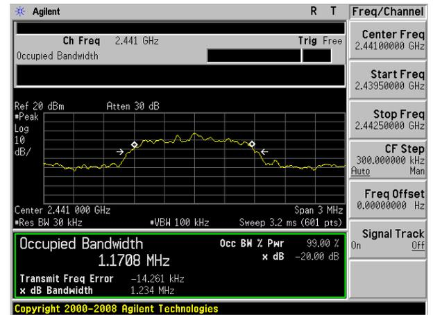
20dB Bandwidth plot on channel 78 (1Mbps)
