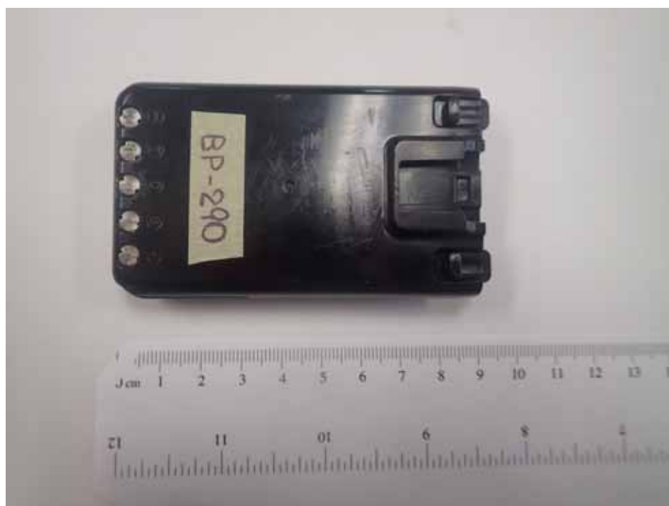
Li-ion Chargeable Battery (M/N: BP-290 Li-ion, 3.7V, 1960mAh)
