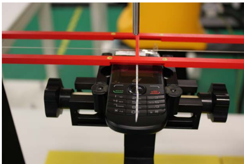
Picture 3: EUT Positioning for T-coil
