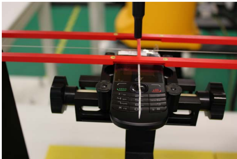
Picture 2: EUT Positioning for RF
