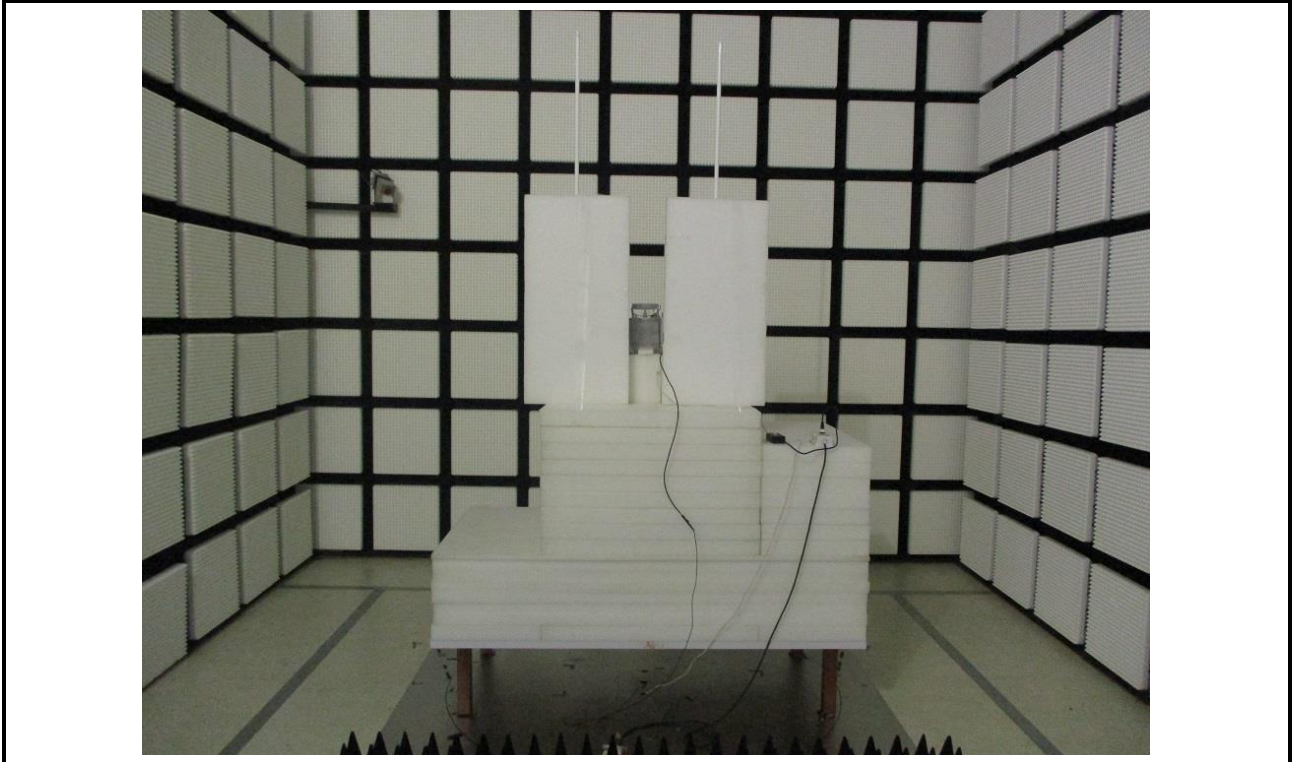
Radiated Emission Above 1GHz Test (POE mode)
