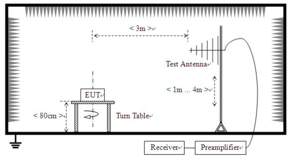
(For the test frequency from 30MHz to1GHz)
