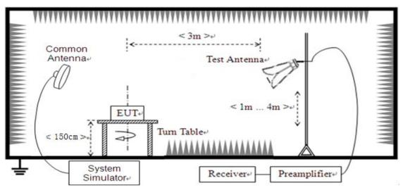
(For the test frequency above 1GHz)
