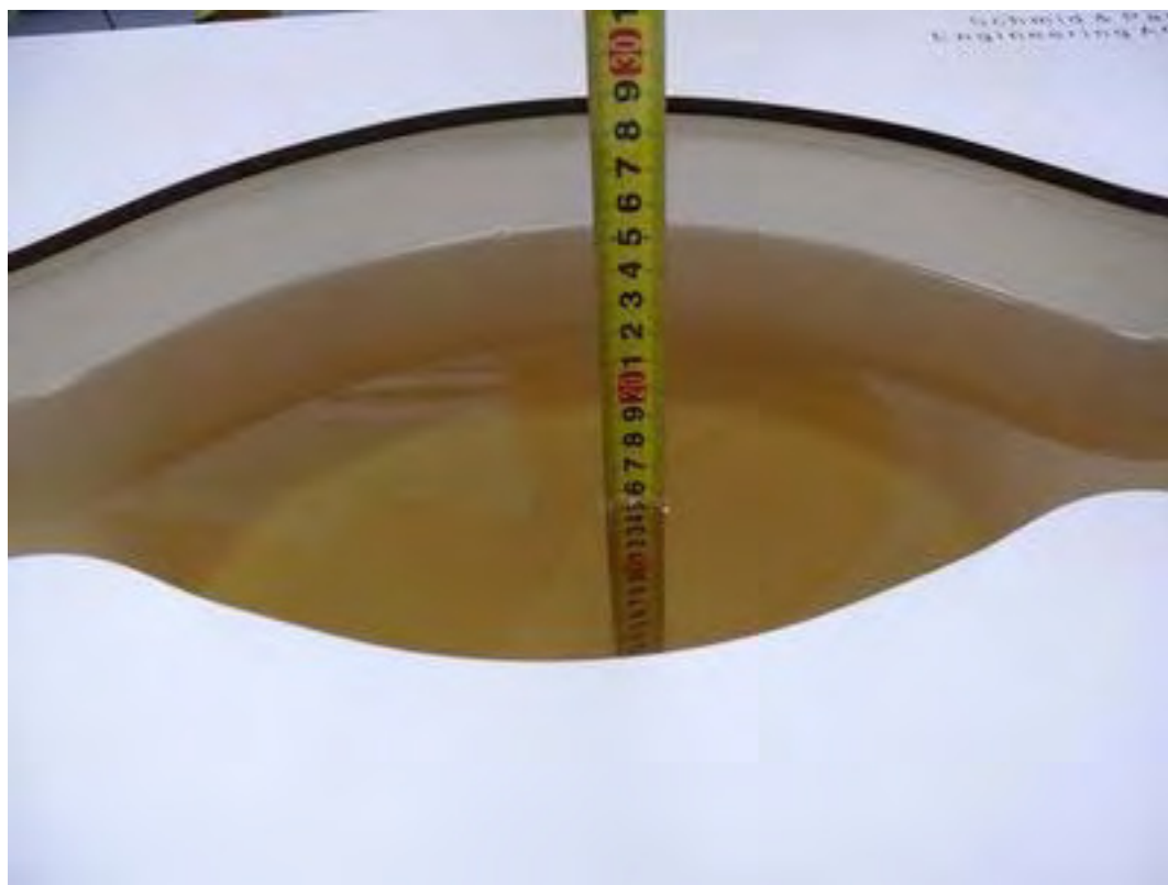
Picture 6: Liquid depth in the flat Phantom (835MHz, 15.4cm depth)
