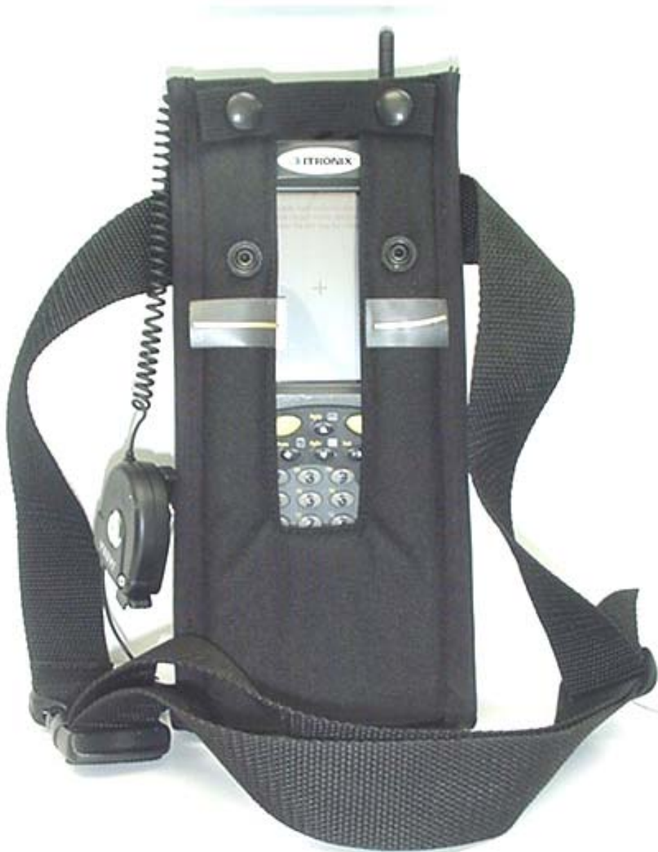
DUT with Nylon Carry Case (P/N: 54-0644-001) & JABRA Ear-microphone
