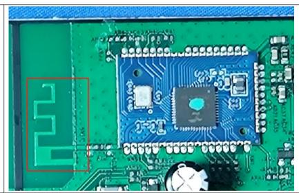
The antenna is PCB antenna.
