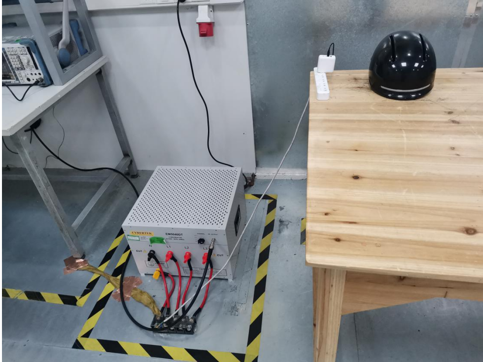
FCC ID: 2A25E-FARO Photo of Conducted Emission Measurement
