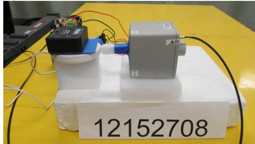
S2, RF EXPOSURE SETUP PHOTO
