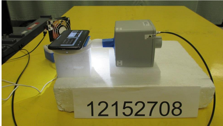
S1, RF EXPOSURE SETUP PHOTO
