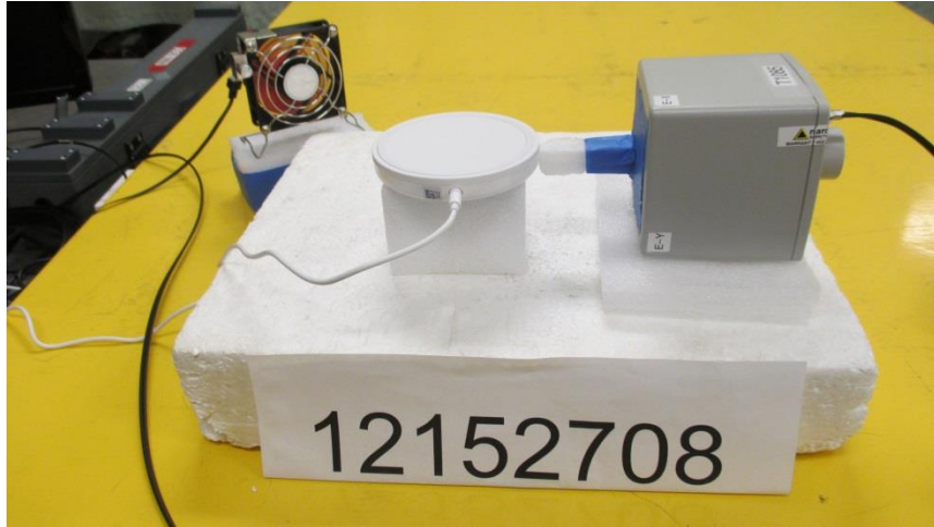
S3, RF EXPOSURE SETUP PHOTO
