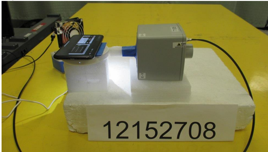
S1, RF EXPOSURE SETUP PHOTO
