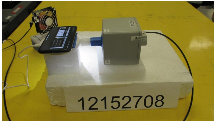
S2, RF EXPOSURE SETUP PHOTO
