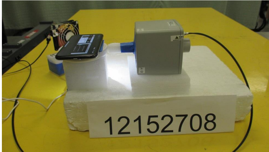
S1, RF EXPOSURE SETUP PHOTO
