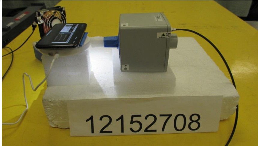
S3, RF EXPOSURE SETUP PHOTO
