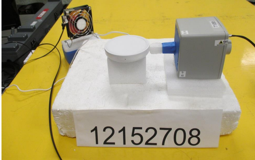
S1, RF EXPOSURE SETUP PHOTO
