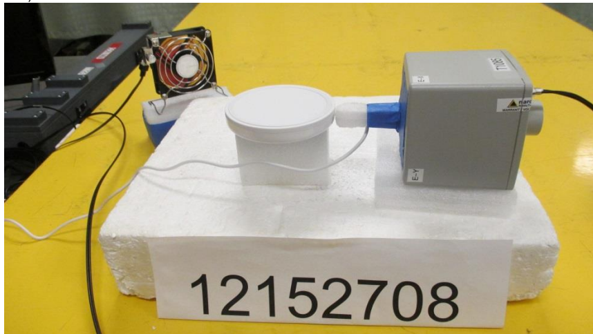
S4, RF EXPOSURE SETUP PHOTO
