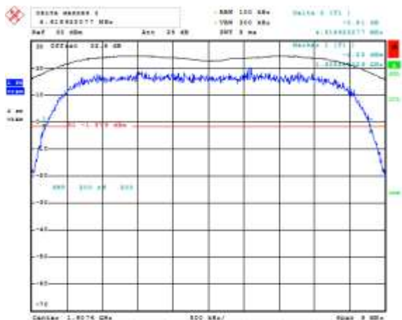
Figure 2-24a: -26 dBc Bandwidth, Band II High Channel
