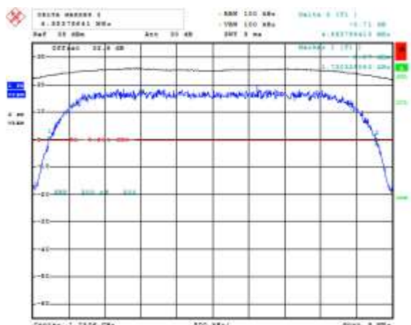
Figure 2-11b: -26 dBc Bandwidth, Band IV Middle Channel
