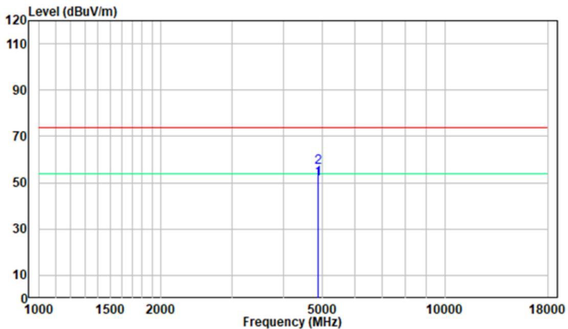
**18-25 GHz (Worst case):****Pre-scan plots for 802.11b Middle Channel****Horizontal**
