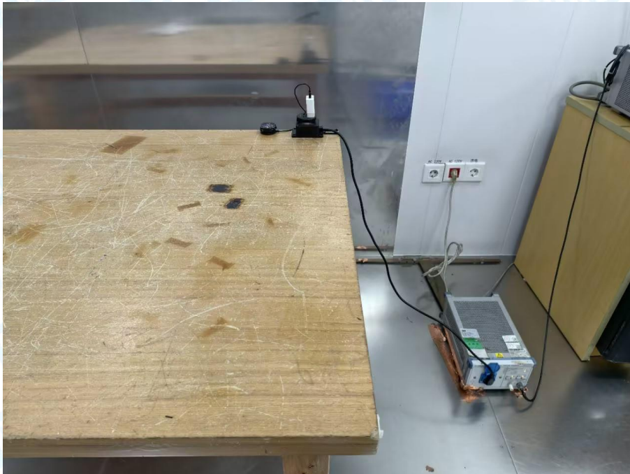
Photo of Setup for Radiated Emission (30MHz~1GHz)
