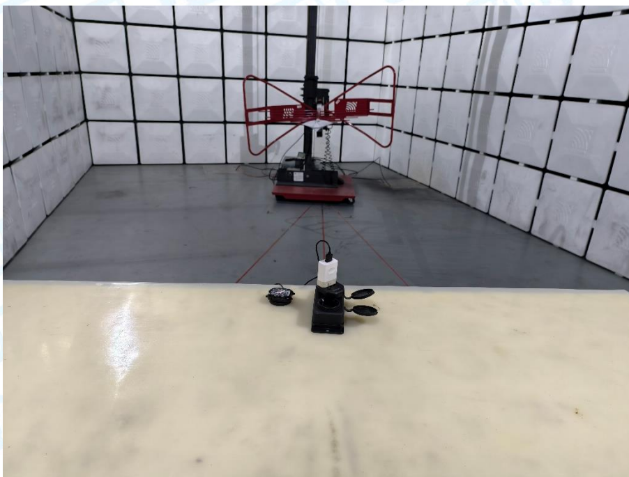
Photo of Setup for Radiated Emission (30MHz~1GHz)
