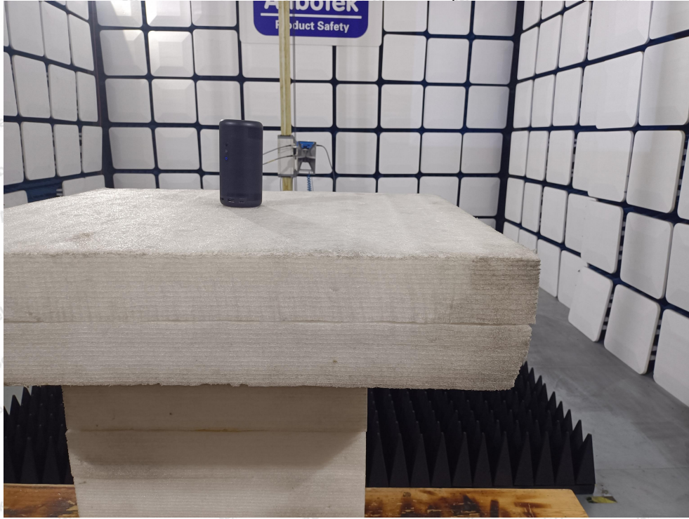
Photo of Radiation Emission Test (above 1GHz)
