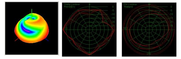
2.4GHz Gain: 2.21dBi Efficiency:64.5%
