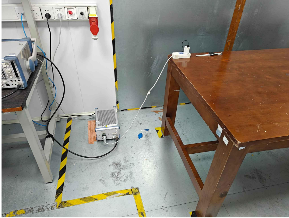
Conducted emissions at AC power line (150kHz-30MHz)
