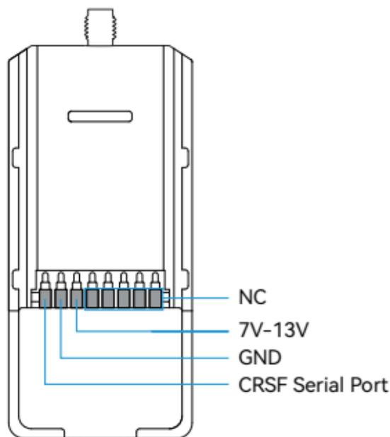
**Note:** Please assemble the antenna before powering on. Otherwise, the PA chip will be damaged permanently.
