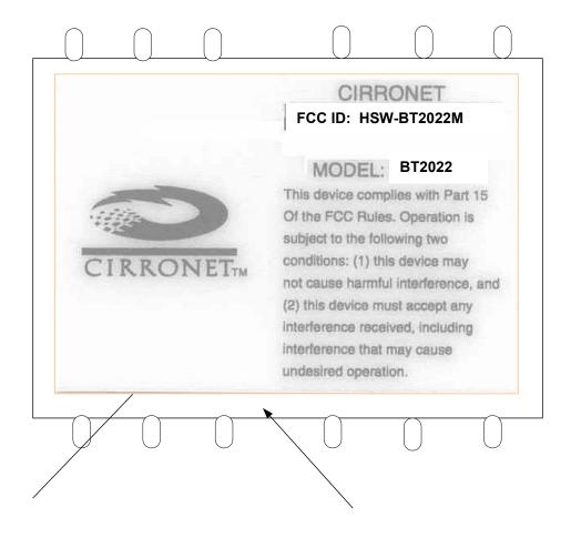
The FCC ID sticker is mounted center on the top shield. The top is defined as the plane with the coax connector facing up.
