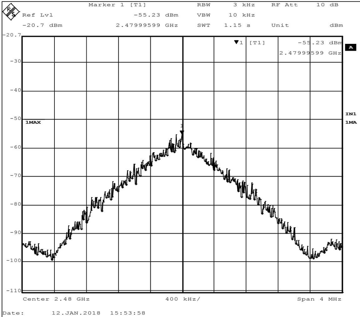
**Figure 20 - Power Spectral Density Measurement, High Channel**
