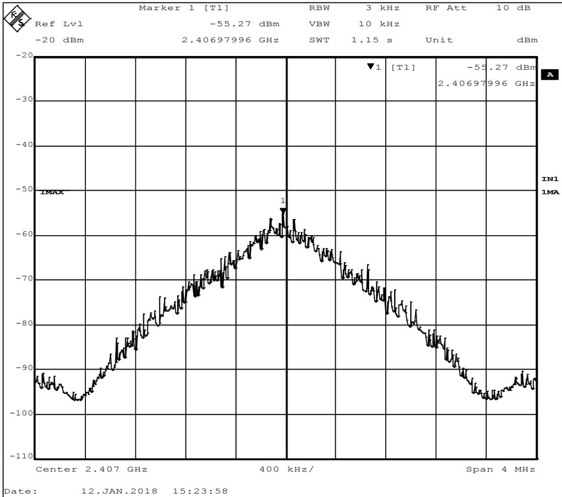
**Figure 18 - Power Spectral Density Measurement, Low Channel**
