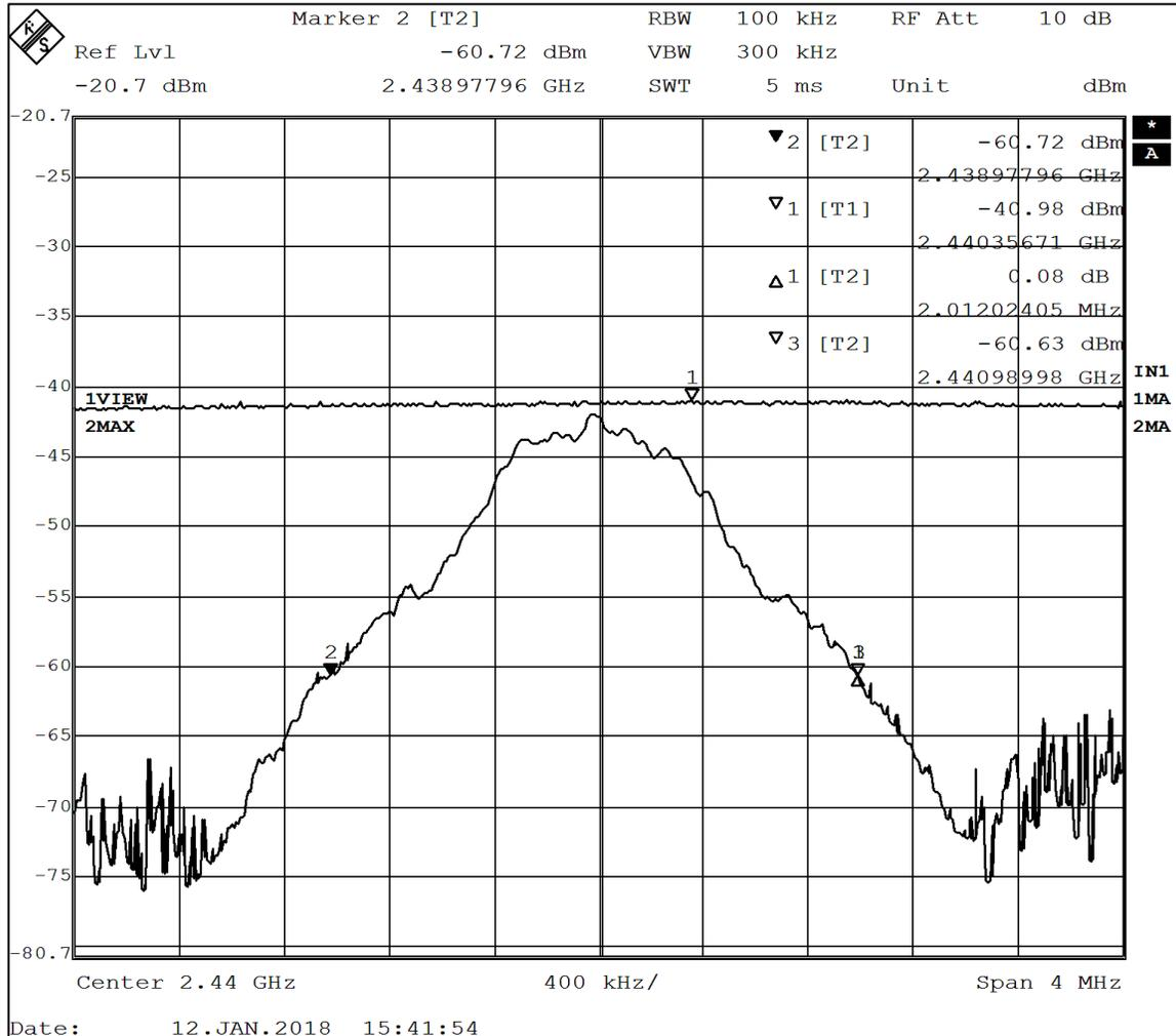
**Figure 8 - 99% Occupied Bandwidth, Mid Channel**
