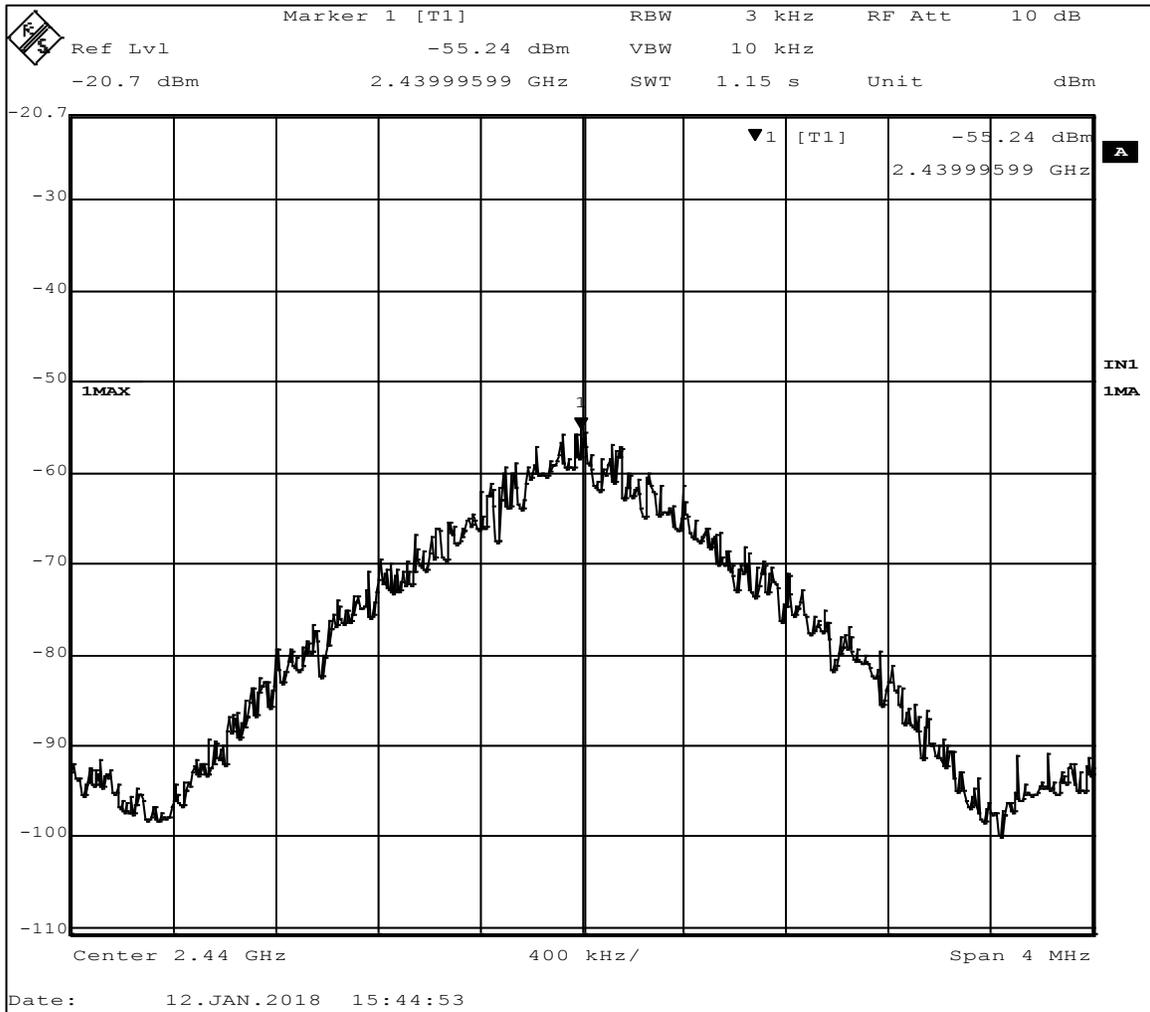
**Figure 19 - Power Spectral Density Measurement, Mid Channel**
