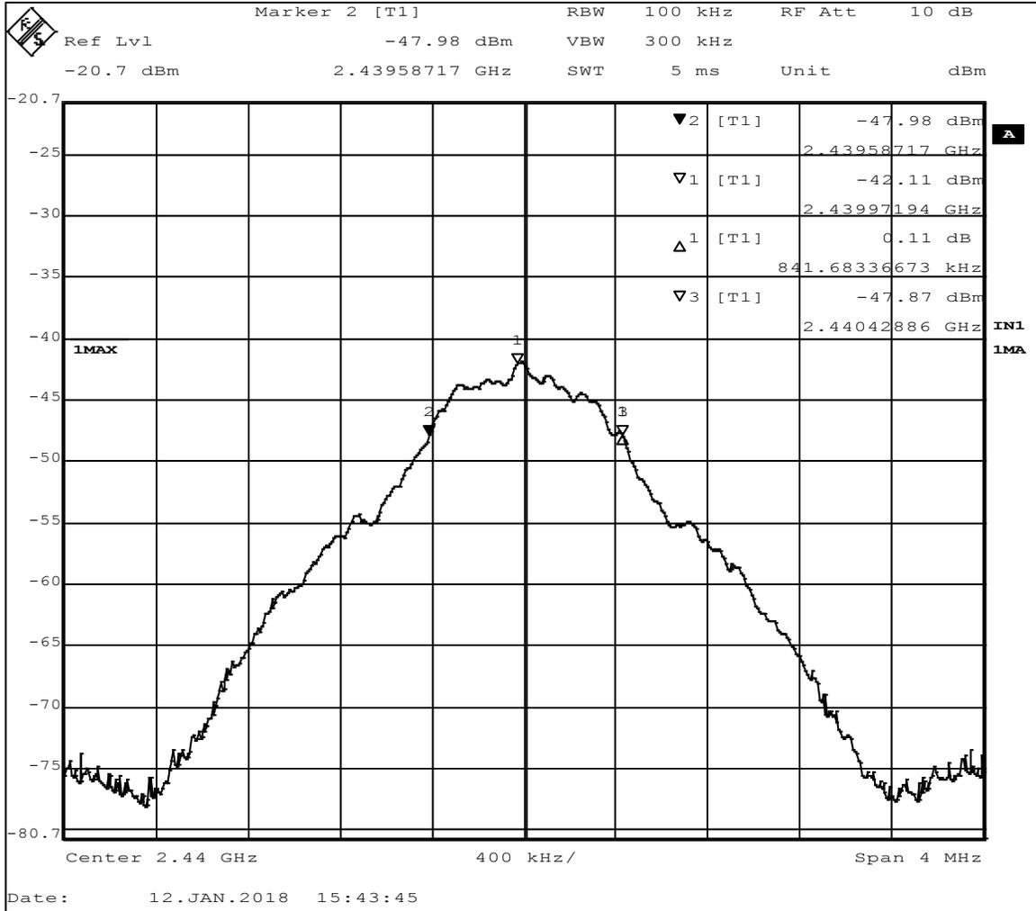
Figure 11 - 6dB Bandwidth, Middle Channel
