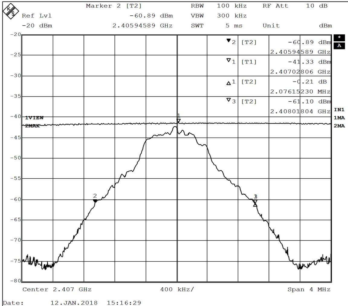
**Figure 7 - 99% Occupied Bandwidth, Low Channel.**
