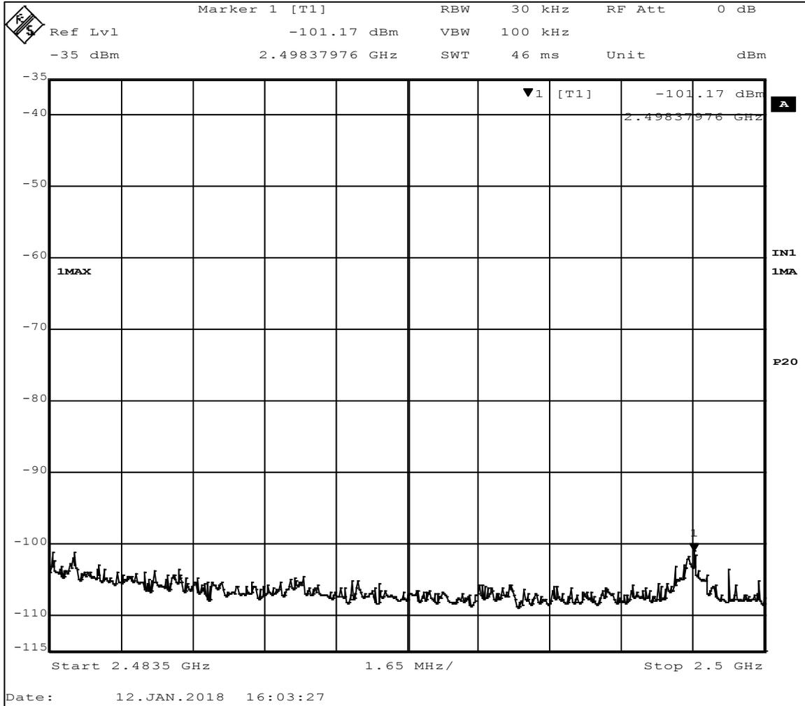
**Figure 16 – Restricted Band-edge Measurement, High Channel, Restricted Frequency**
