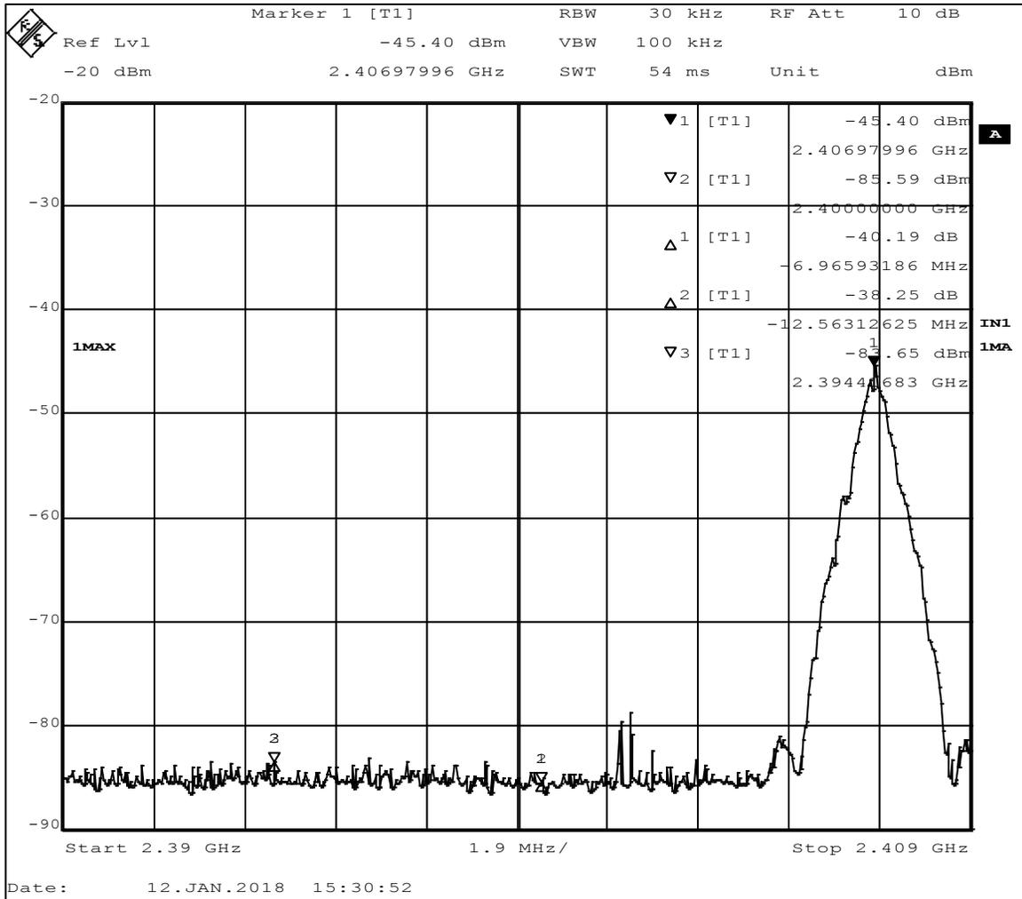
**Figure 14 – Restricted Band-edge Measurement, Low Channel, Fundamental**
