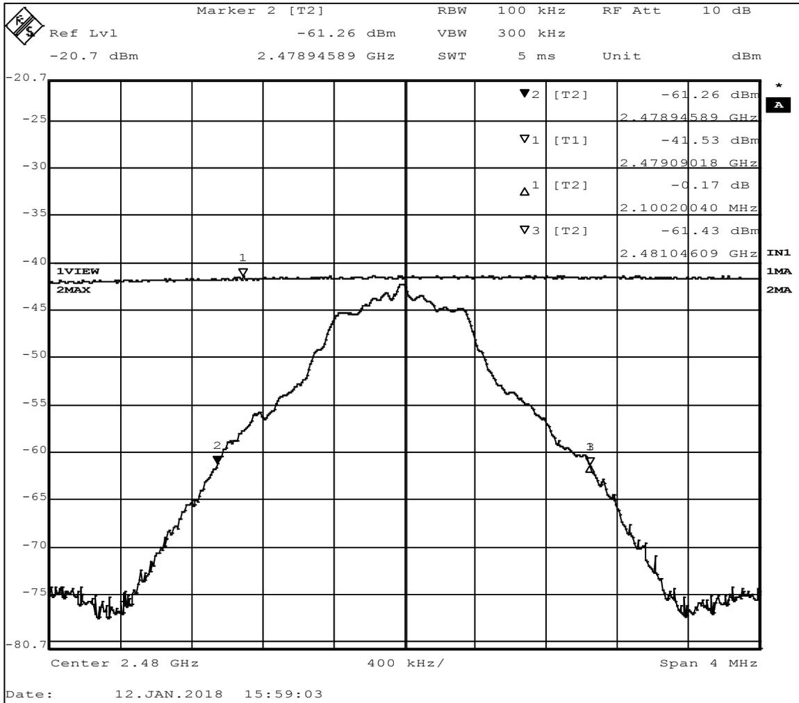
Figure 9 - 99% Occupied Bandwidth, High Channel
