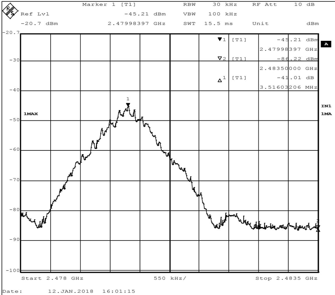
**Figure 17 - Band-edge Measurement, High Channel, Fundamental**
