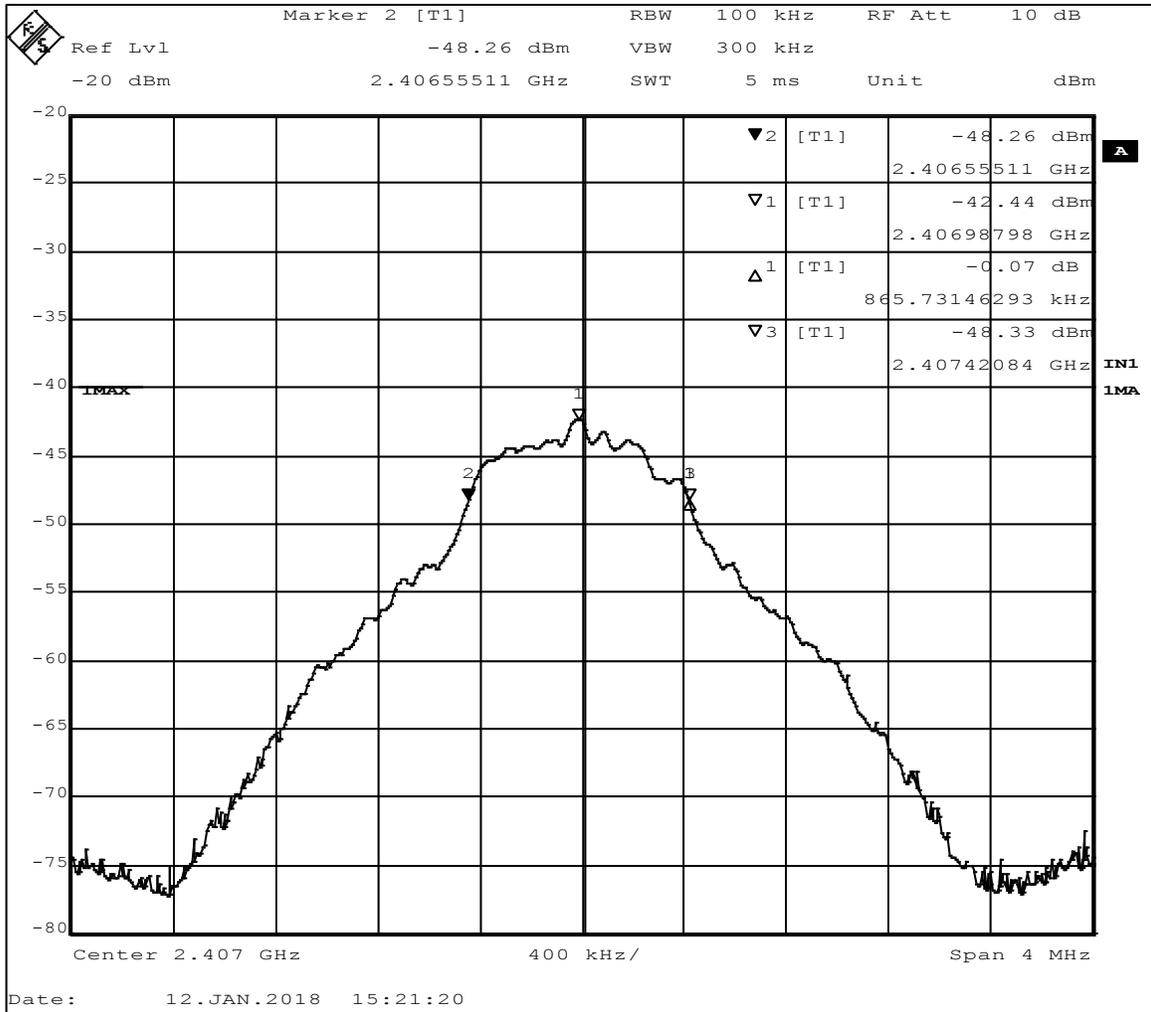
Figure 10 - 6dB Bandwidth, Low Channel
