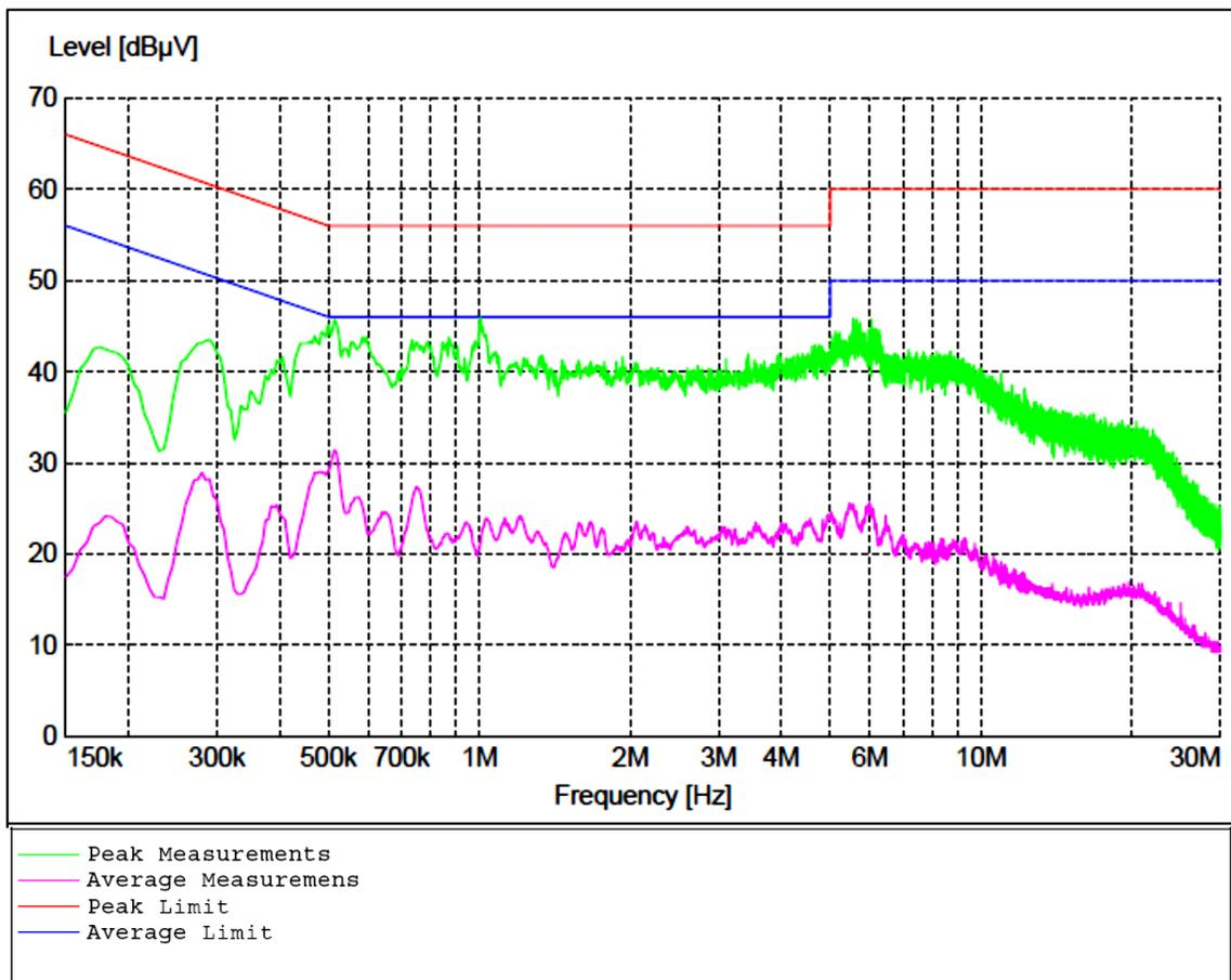
**Figure 21 - Conducted Emissions Plot**
