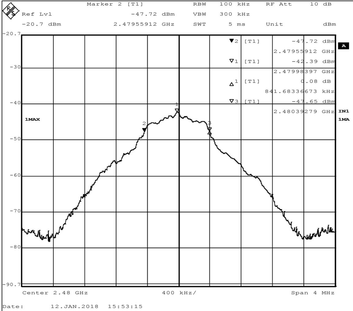
Figure 12 - 6dB Bandwidth, High Channel
