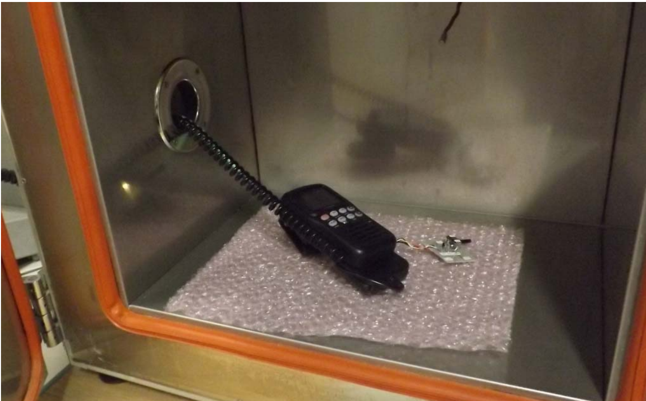
Figure E23.4 – Setup, Frequency Stability
