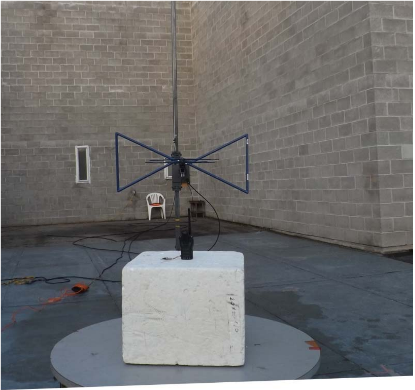
Figure E23.5 – Setup, Radiated Measurements Below 1GHz
