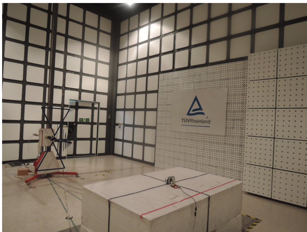
Photograph 2: Set-up for Spurious Emissions (Back View 1)
