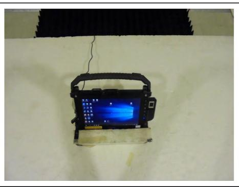
Description: Back View of Radiated Emission Test \_ Above 1 GHz
