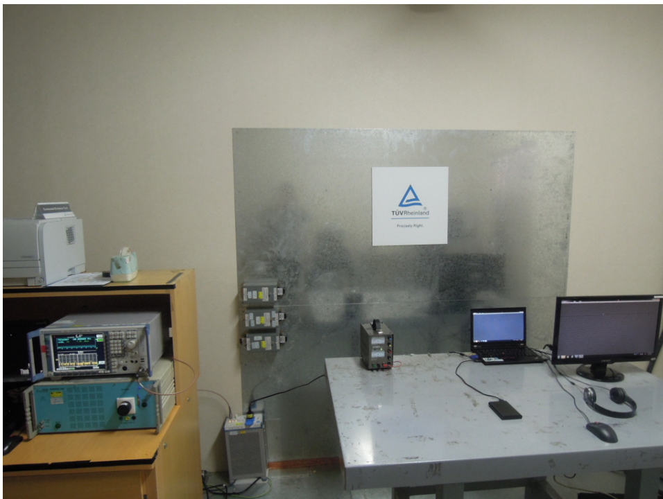
Photograph 8: Set-up for Mains Conducted testing (Front View)
