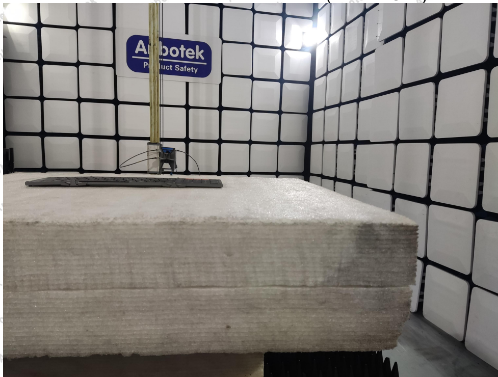
Photo of Radiation Emission Test (above 1GHz)
