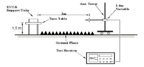
The radiated emission below 1GHz tests were performed in the 10 meters chamber test site, above 1GHz tests were performed in the 3 meters chamber test site B, using the setup accordance with the ANSI C63.10-2013. The specification used was the FCC 15.209, and FCC 15.247 and the RSS-247 Clause 5.5, RSS-GEN Clause 8.10 limits.
