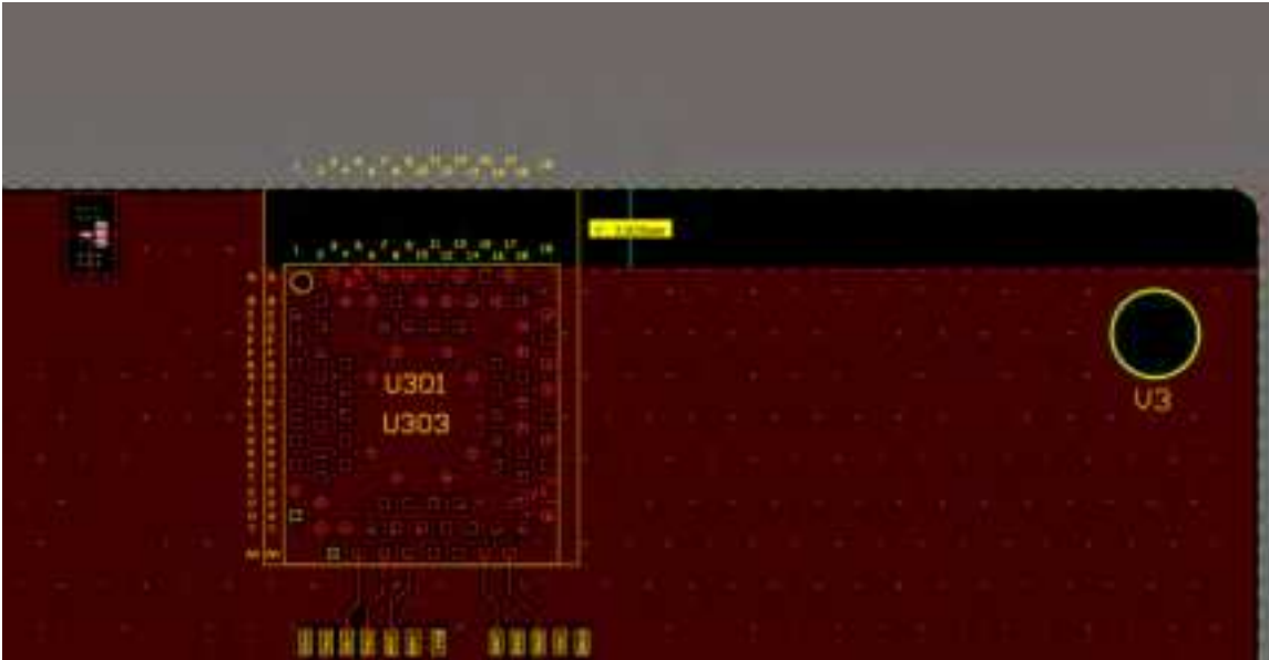
Figure 11: WE310F5-I Placement Example showing no copper in any layer of the board.
