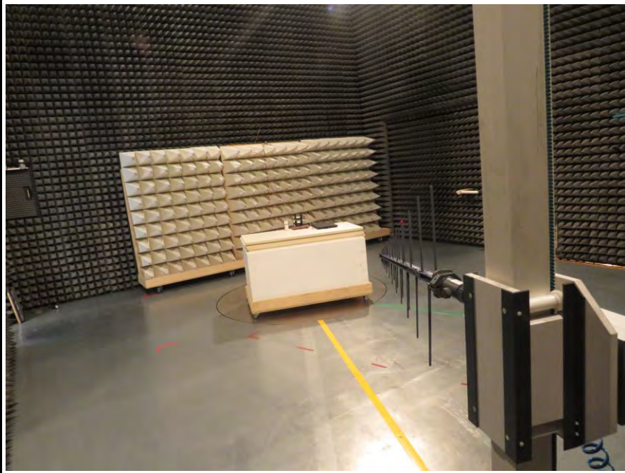
Setup for measurements below 1 GHz for Variant 2 (NORA-W101 with external antenna PN PRO-IS-237)
