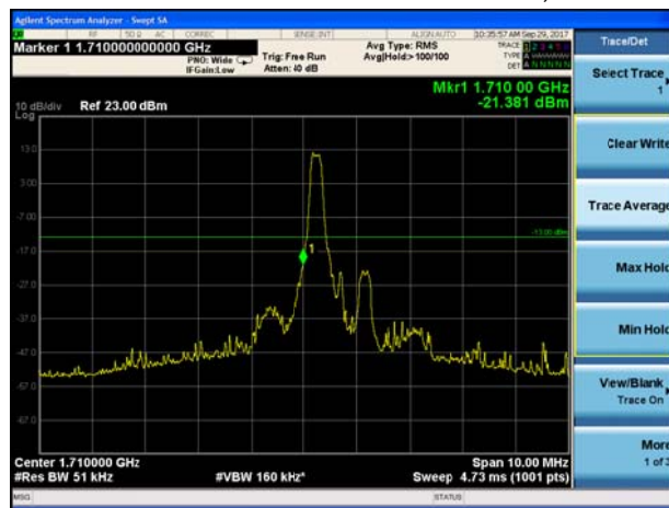
LTE Band 4 QPSK 1.4MHz CH-Low, 100%RB
