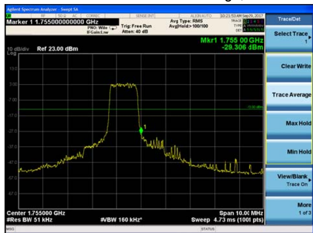
LTE Band 4 QPSK 3MHz CH-High, 1 RB
