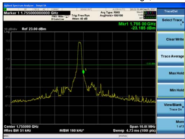
LTE Band 4 QPSK 1.4MHz CH-High, 100%RB
