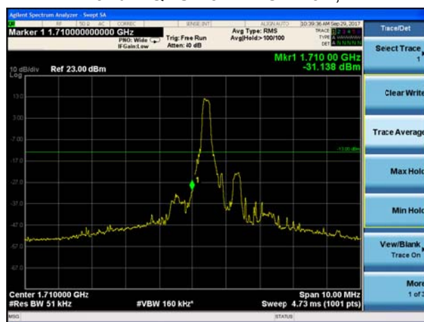
LTE Band 4 QPSK 3MHz CH-Low, 1 RB
