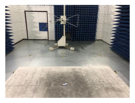
RADIATED EMISSION TEST SETUP ABOVE 1GHZ
