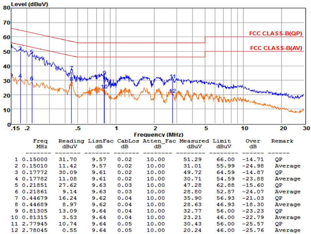
Remarks: 1. Measured = Reading + Lisn Factor +Cable Loss+Atten\_Fac.
