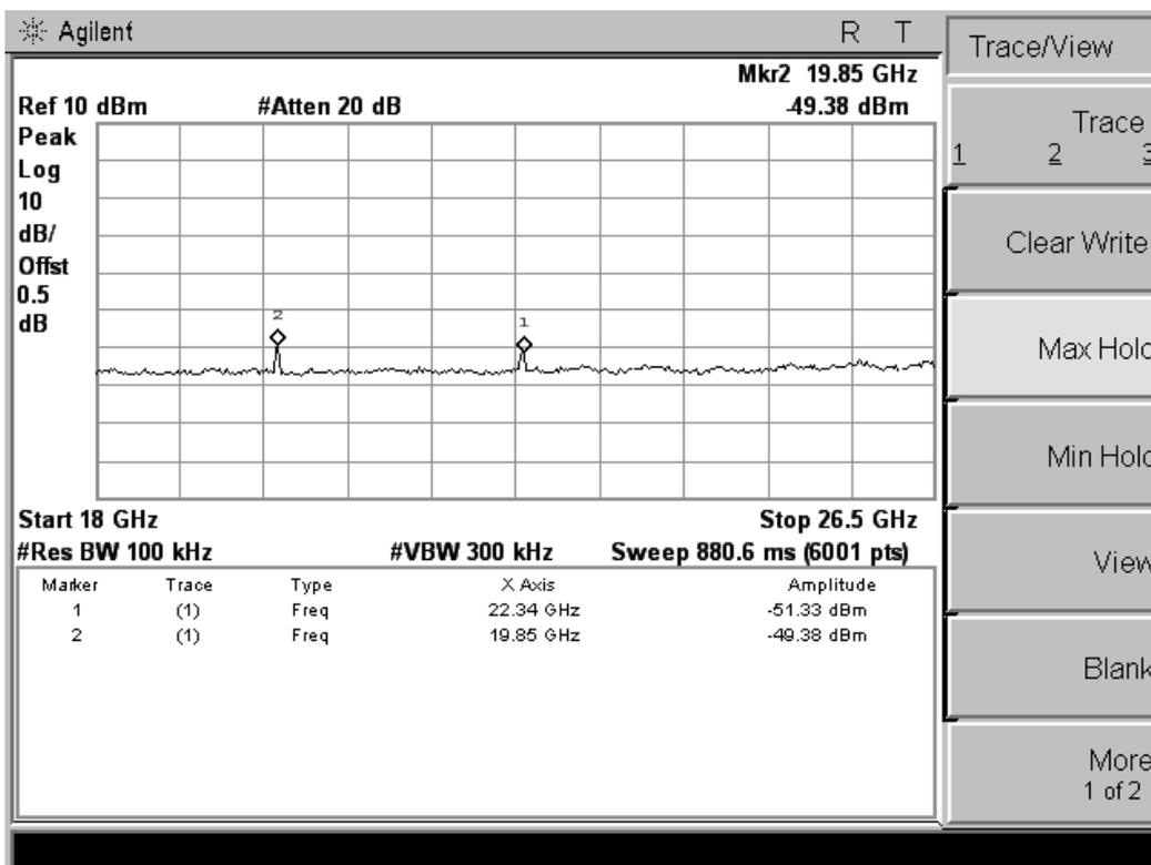
5.6.7. Test Results of Band Edges Test
