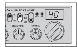
**1** Switch to BRT or DIM to control the brightness of the channel indicator and multi-function meter for day or nighttime driving.
