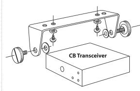
2 Drill the holes and secure the bracket.
