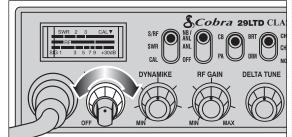
3 To achieve the Desired Squelch Setting (DSS), turn the Squelch control © counterclockwise until you hear noise. Now turn the control clockwise just until the noise stops. This is the DSS setting.
