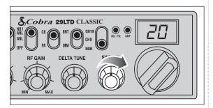
While holding the mic button adjust the SWR CAL knob so the meter needle swings to the CAL ▼ mark on the right side of the meter.
