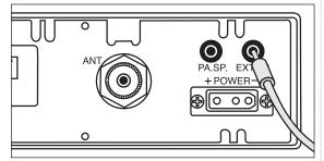
Connect an external speaker to the external speaker jack on the rear panel.
