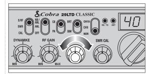
• Rotate Delta-Tune knob to the center position for optimum tuning.
