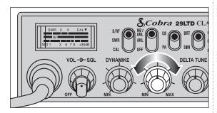
• Rotate the © RF Gain knob counterclockwise to reduce gain in strong signal areas. In weak signal areas turn clockwise to increase the gain.
