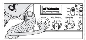
Attach the 4-pin microphone cable to the connector on the front of the radio and install the microphone on bracket securely.
