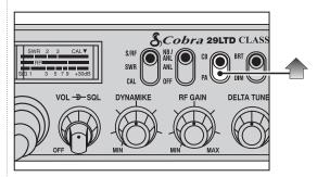
**1** The <sup>®</sup> CB/PA button should be in the CB position.
