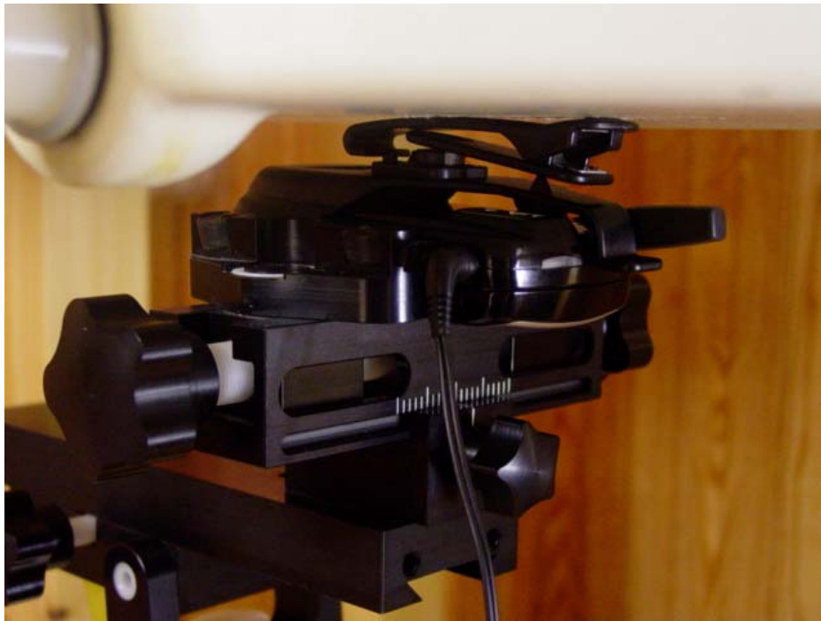
Figure 12.6 body SAR setup (with holster)
