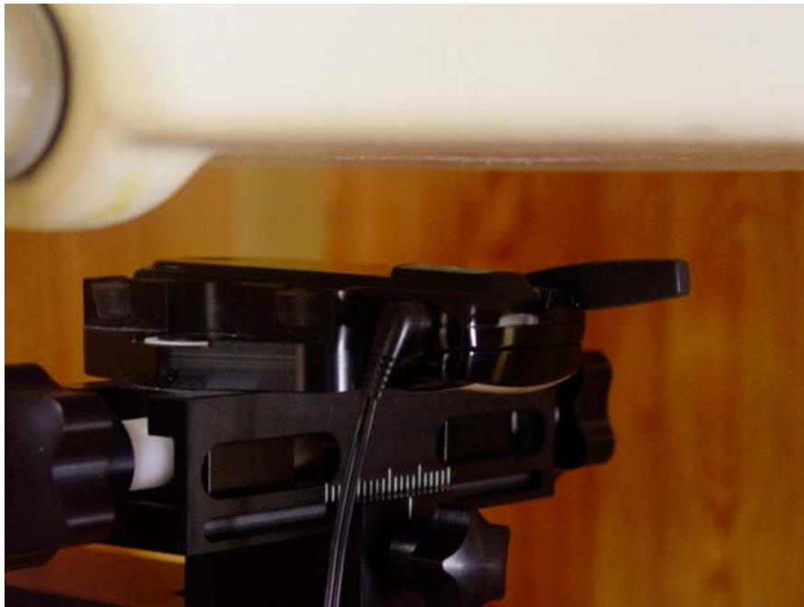
Figure 12.8 body SAR setup (with 25mm air separation)
