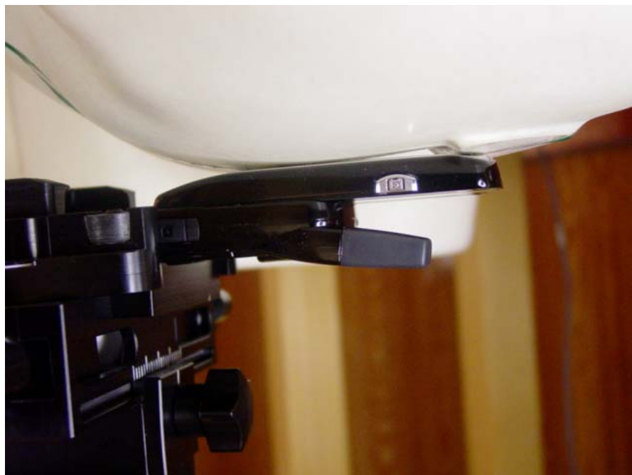
Figure 12.1 phone against the head (left cheek closed position)
