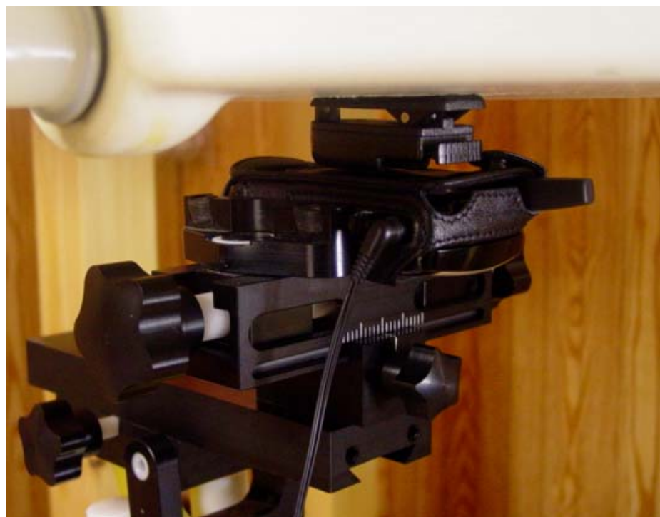
Figure 12.7 body SAR setup (with leather case)
