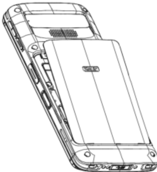
Fig. 5-1 Load the battery
