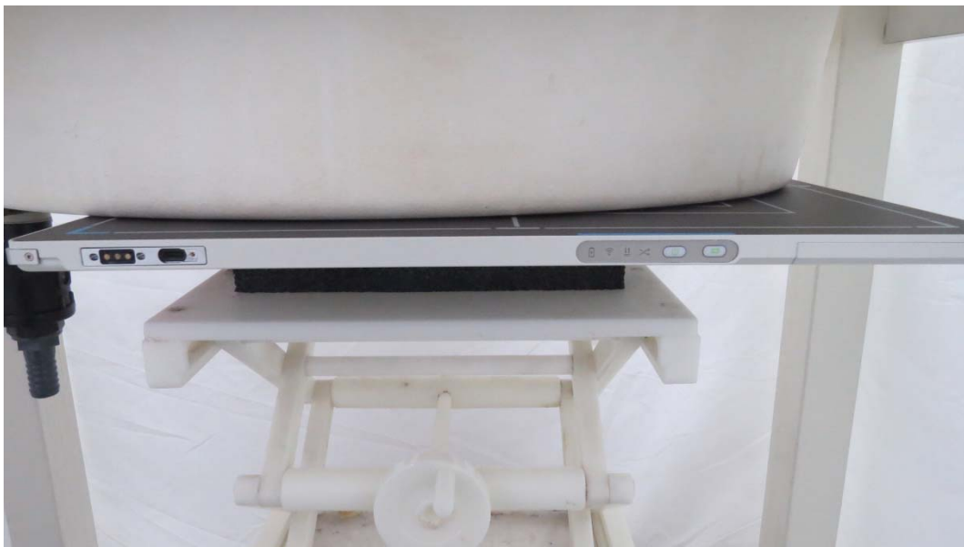
Picture 8: Front Side, the distance from handset to the bottom of the Phantom is 0mm (Scan 4)
