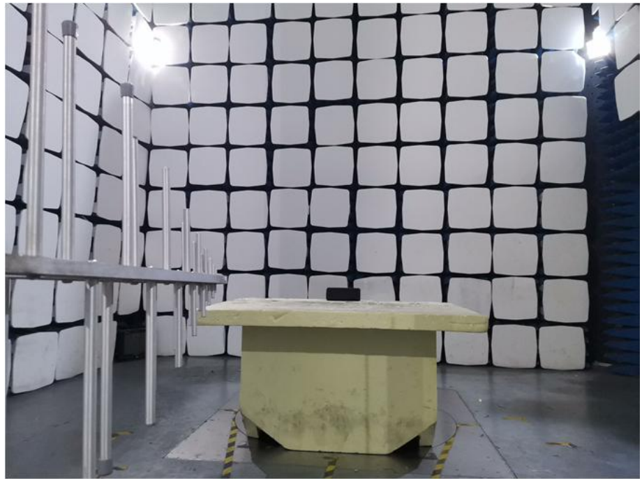
Radiation Emission Test Setup (30MHz to 1GHz)
