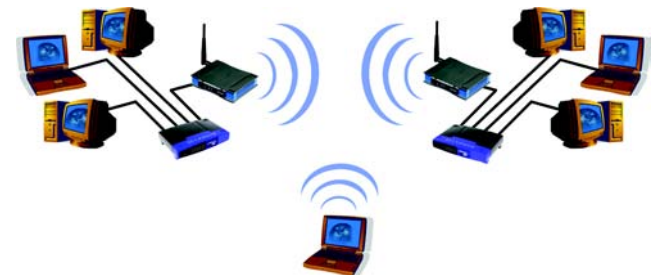
Figure 2-3: Network Using Wireless Bridging
