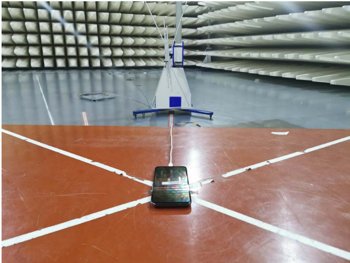
Spurious Radiated Emissions Test setup
