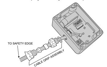
STEP 6 Attach Cable. Attach safety edge cable to terminals as shown. Tighten cable grip assembly using pliers to assure a water tight seal.
