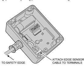
DTG Code Setting. To set a code, select any valid combination of ON and OFF positions for the switch keys numbered 1 - 8. Refer to receiver installation instructions to code receiver switches.
