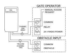
Test System. Activate the gate to close. As the gate is closing, press the safety edge with your hand. Gate should stop and reverse.
