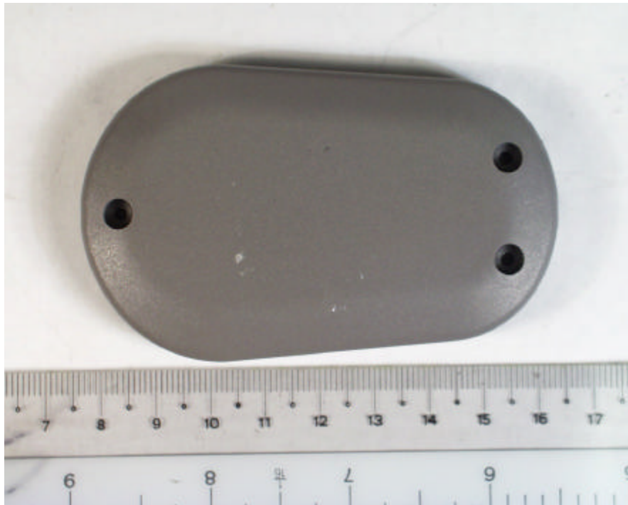
Bottom Housing External View – RF Dongle
