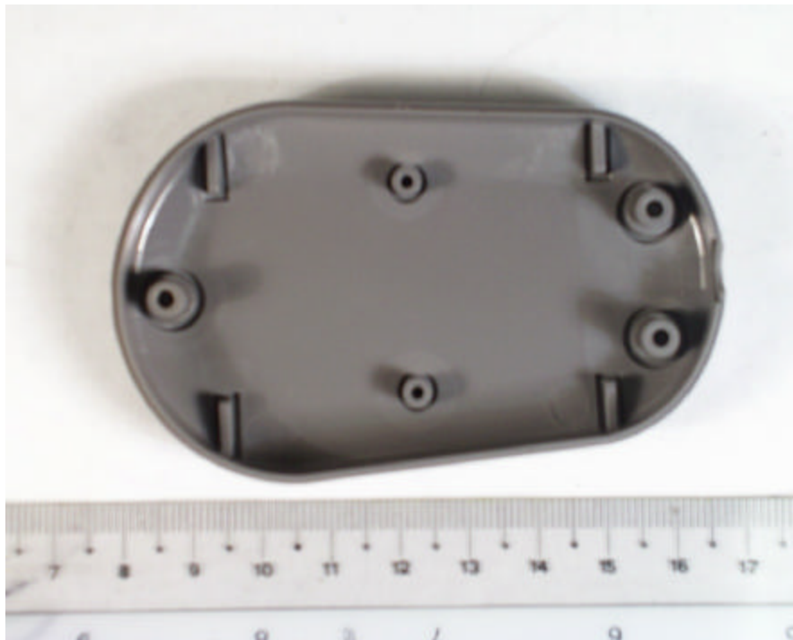
Bottom Housing Internal View – RF Dongle
