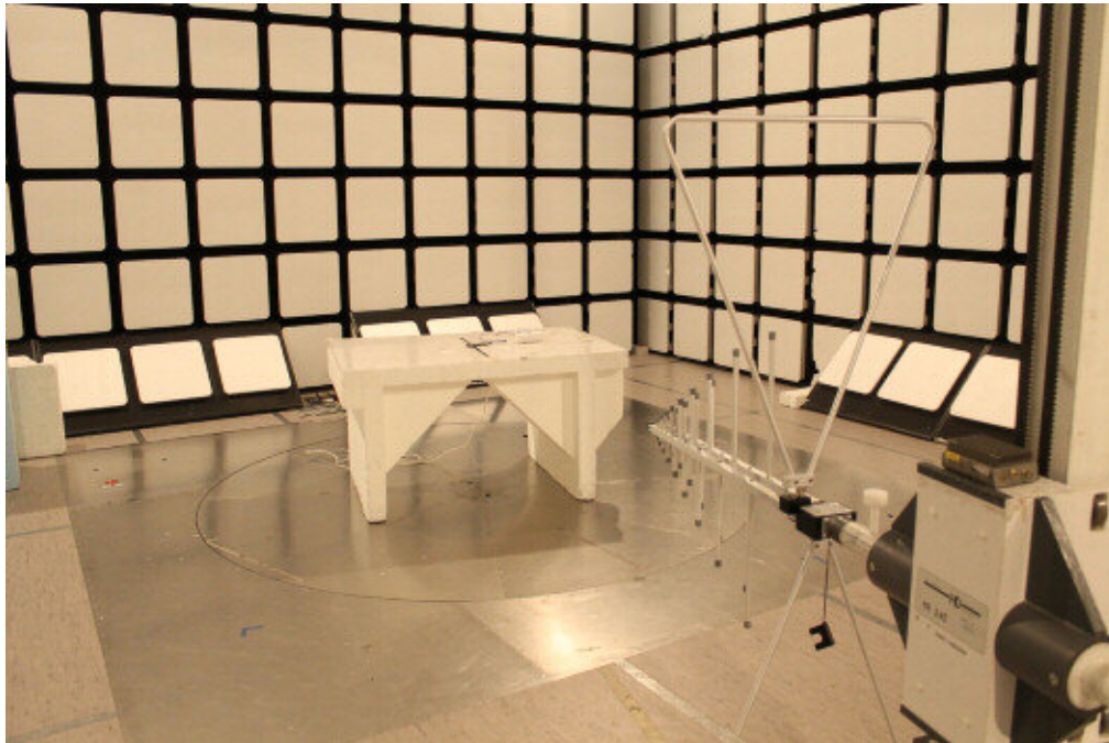
Photograph 1. Radiated Spurious Emissions 30 – 1000 MHz
