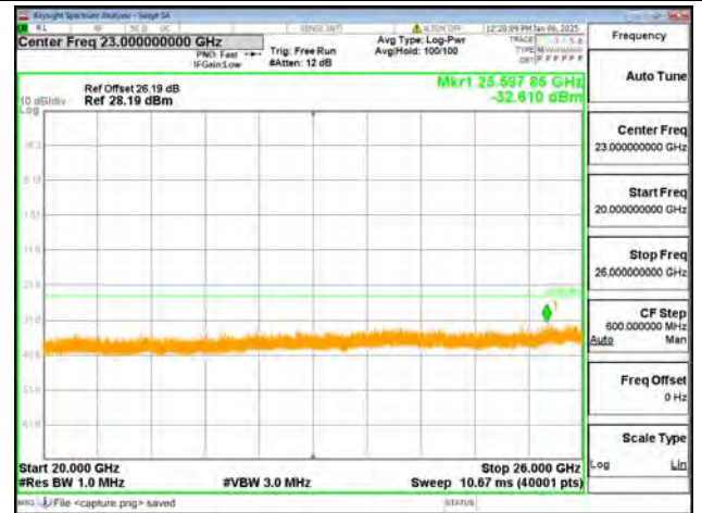
B7-20G-26G / 15MHz / Mid CH / QPSK
