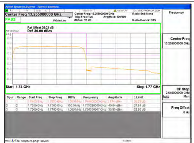
B4 / 15MHz / High CH / QPSK / FULL RB
