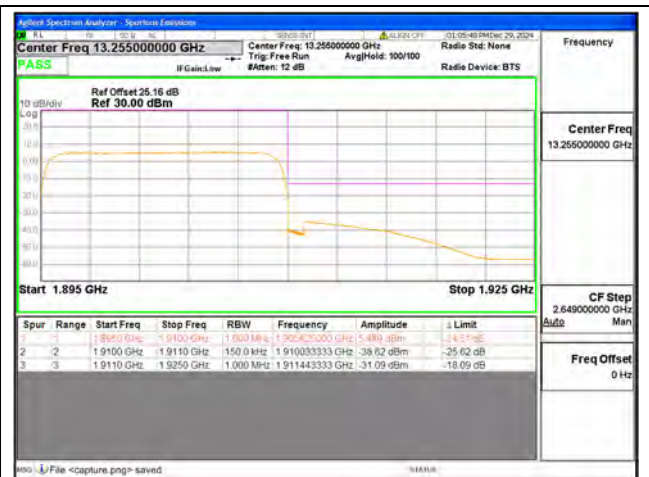
B2 / 15MHz / High CH / QPSK / FULL RB
