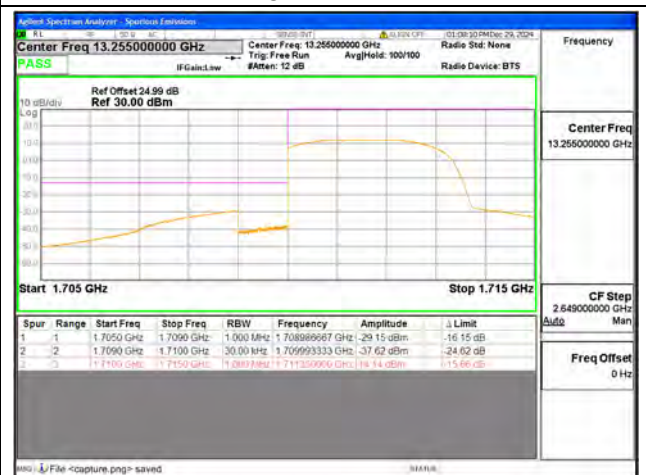
B4 / 3MHz / Low CH / QPSK / FULL RB
