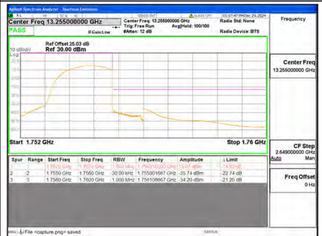
B4 / 1.4MHz / High CH / QPSK / FULL RB
