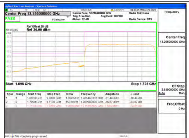
B4 / 15MHz / Low CH / QPSK / FULL RB
