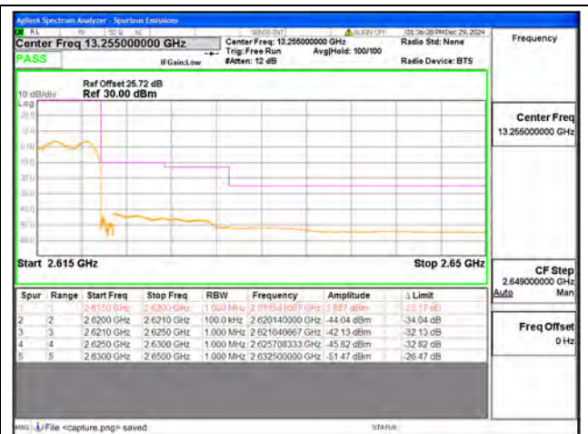
B38 / 10MHz / High CH / QPSK / FULL RB
