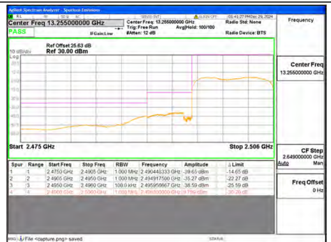
B41 / 10MHz / Low CH / QPSK / FULL RB
