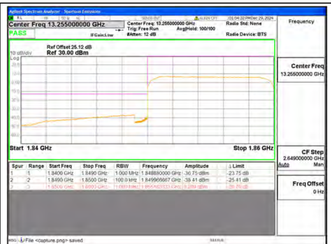
B2 / 10MHz / Low CH / QPSK / FULL RB
