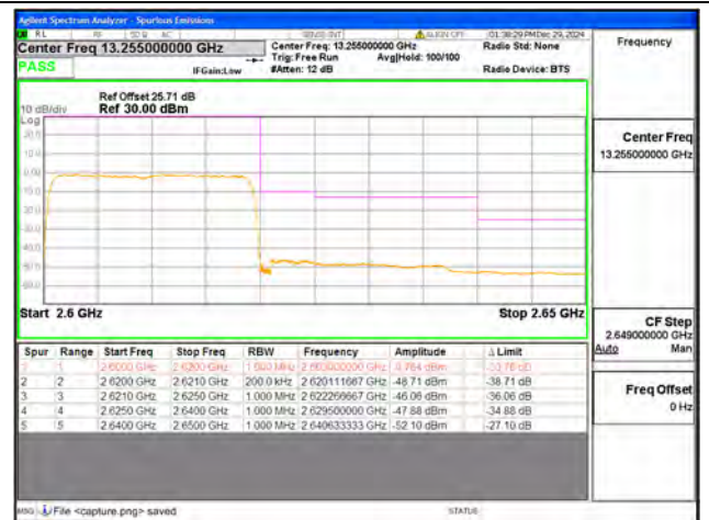
B38 / 20MHz / High CH / QPSK / FULL RB
