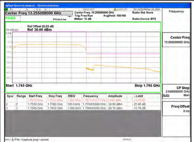
B4 / 10MHz / High CH / QPSK / FULL RB
