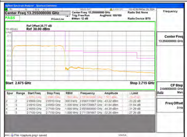
B41 / 15MHz / High CH / QPSK / FULL RB
