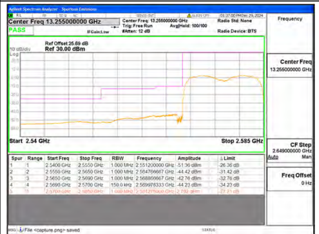
B38 / 15MHz / Low CH / QPSK / FULL RB
