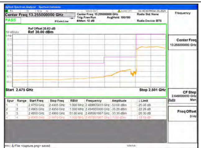
B41 / 5MHz / Low CH / QPSK / FULL RB
