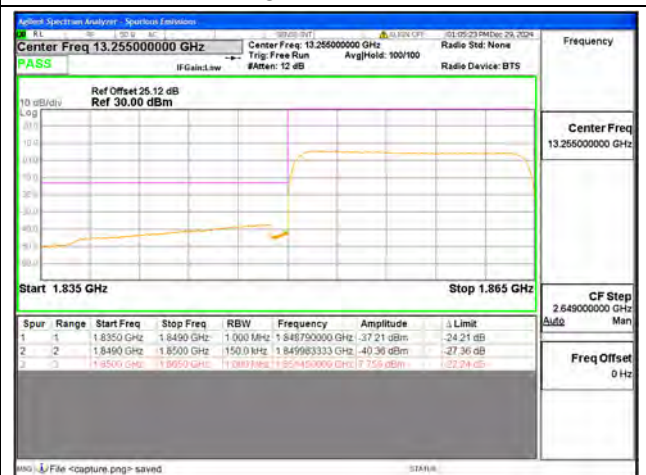
B2 / 15MHz / Low CH / QPSK / FULL RB
