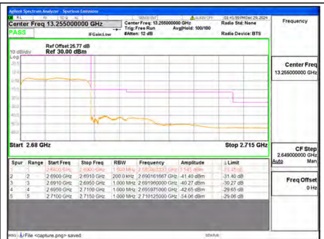
B41 / 10MHz / High CH / QPSK / FULL RB
