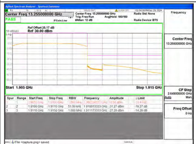
B2 / 5MHz / High CH / QPSK / FULL RB
