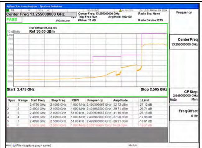
B7 / 5MHz / Low CH / QPSK / FULL RB
