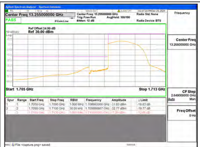
B4 / 1.4MHz / Low CH / QPSK / FULL RB
