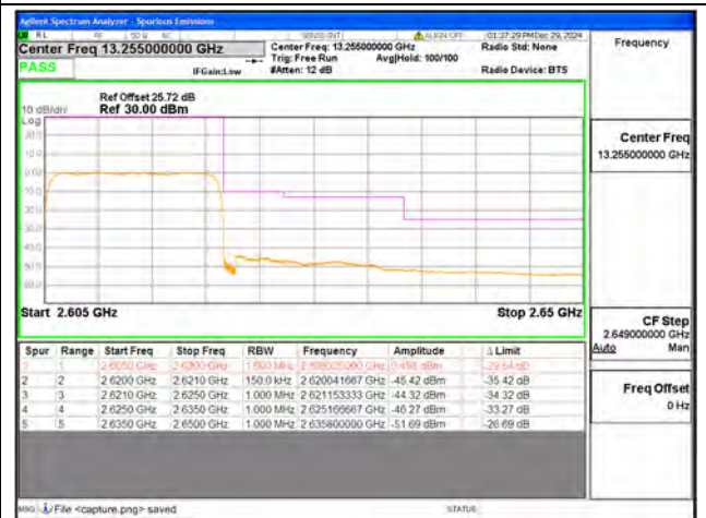
B38 / 15MHz / High CH / QPSK / FULL RB
