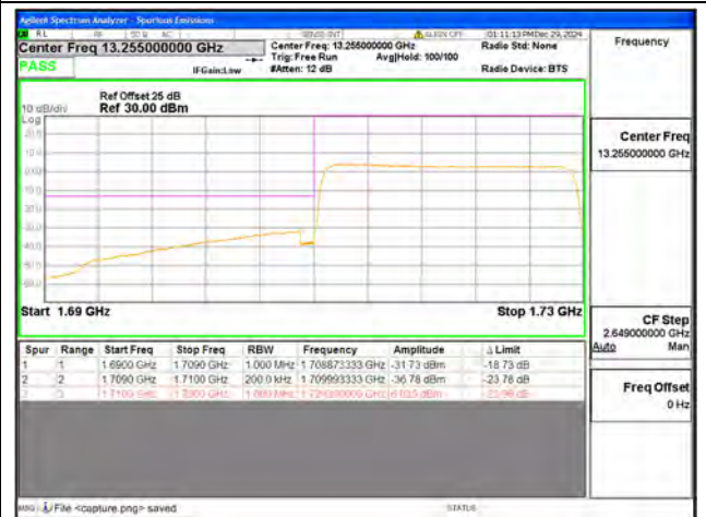
B4 / 20MHz / Low CH / QPSK / FULL RB
