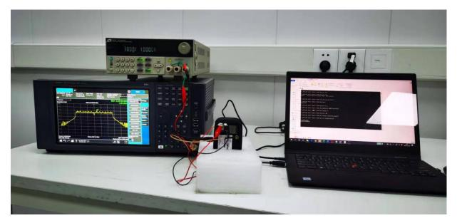
1.2 Set-up for Spurious Emissions below 1GHz
