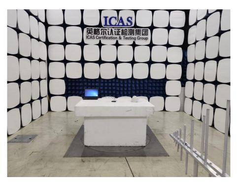
1.3 Set-up for Spurious Emissions above 1GHz
