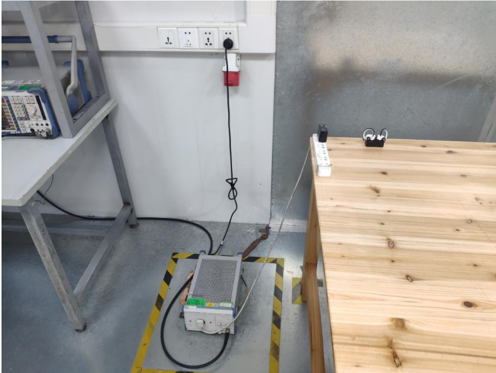
Photo of Conducted Emission Measurement
