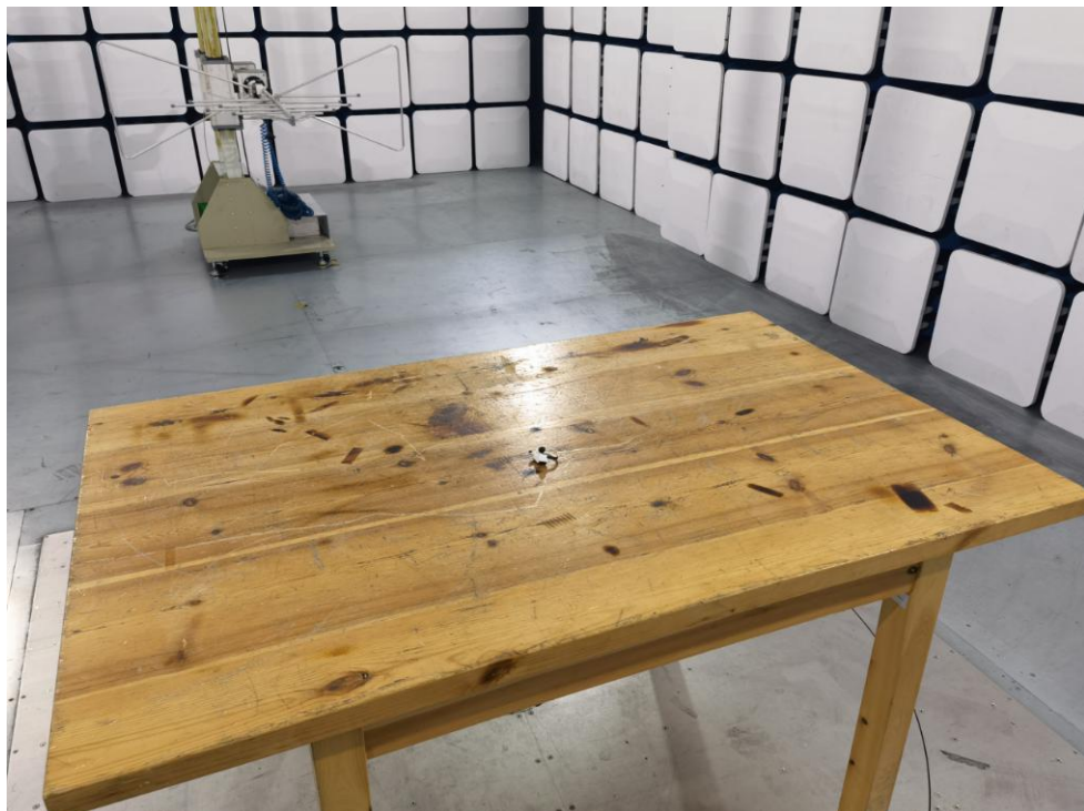
Photo of Radiation Emission Test
