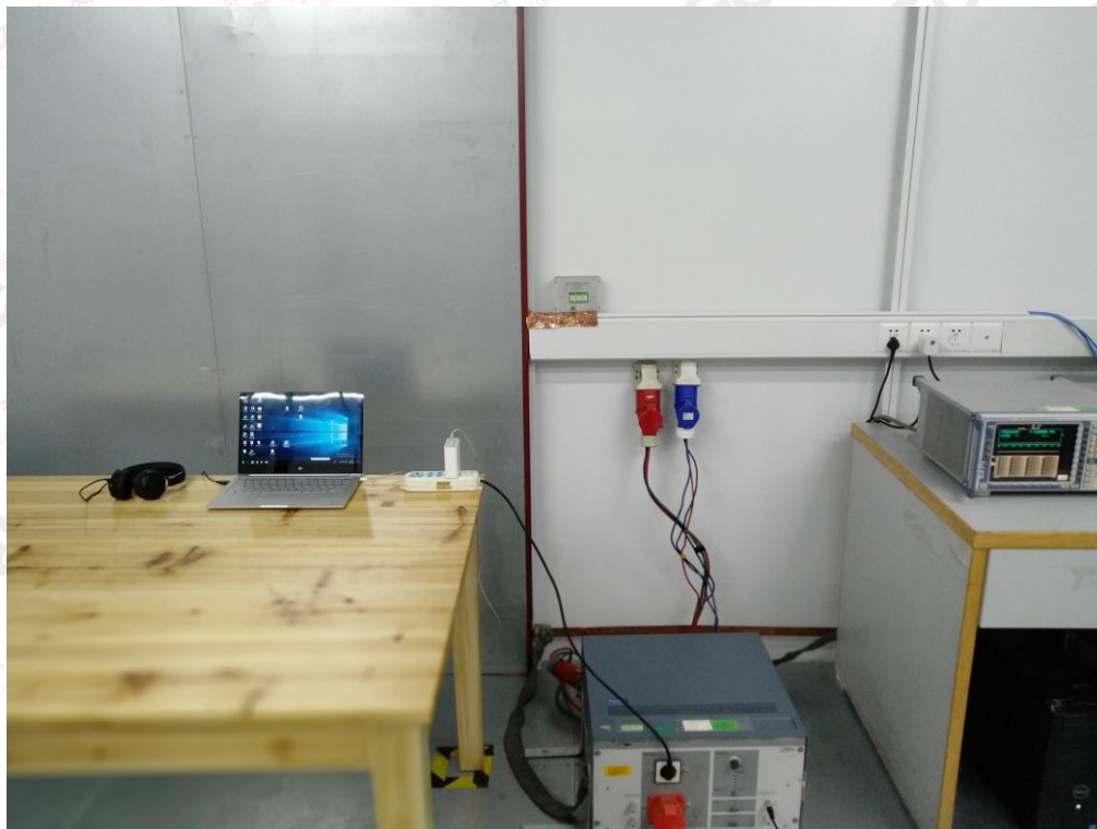
RADIATED EMISSION TEST SETUP
